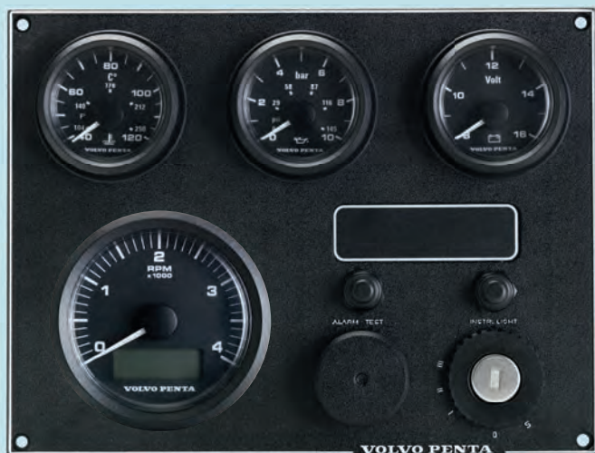
Main station panel with the tachometer (option).
