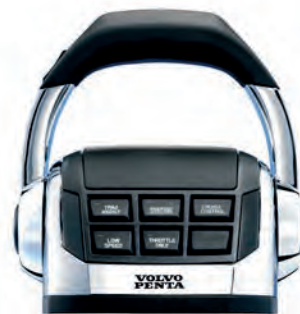
EVC top mount controls, single engine
