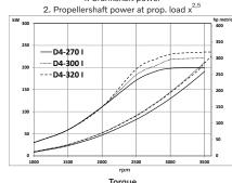
Torque Torque measured at crankshaft -D4-270 -- D4-300 I -- D4-320 I
